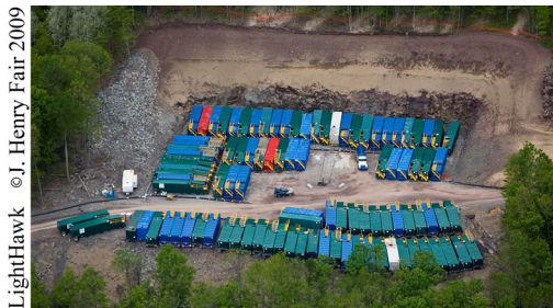
Liquid Stored at Well Site for Fracking
